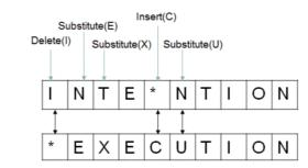
Figure 5-6 Three types of operations in Levenshtein Distance
