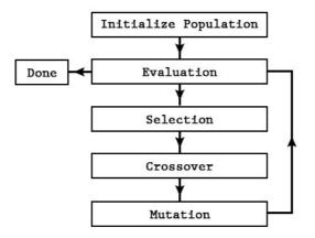
Figure 5-7 A flow chart of the Genetic Algorithm
